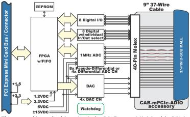
This manual is applicable to both the PCI Express Mini Card (mPCle) and M.2 card versions of this product. The registers, I/O and performance specifications are the same.
